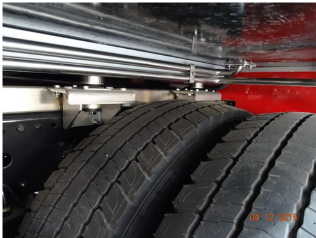
Stainless steel subframe, stainless steel water pipe
