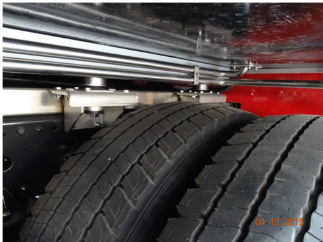
Stainless steel subframe stainless steel water pipe
