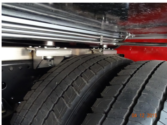
Stainless steel subframe, stainless steel water pipe
